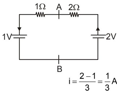
So, P.D. between A & B at steady state  $= 1 + \frac{1}{3} = \frac{4}{3} \text{ V}$
