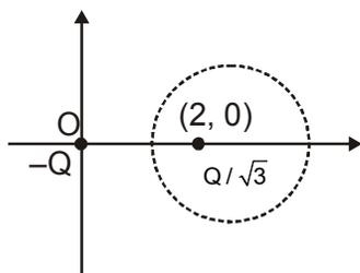
For equipotential circle in  $x - y$  plane, potential should be zero.
