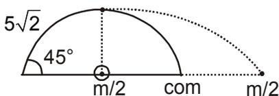
both will take same time to hit the ground as both have same zero initial velocity and same acceleration in vertical direction.
